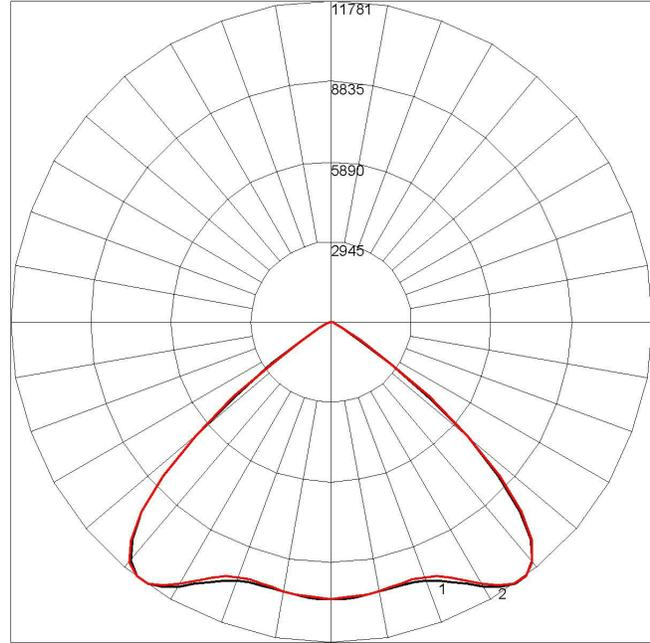
Maximum Candela = 11780.5 Located At Horizontal Angle = 90, Vertical Angle = 37.5
