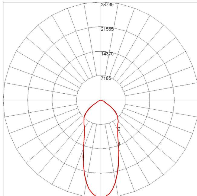
Maximum Candela = 28739.4 Located At Horizontal Angle = 0, Vertical Angle = 0
