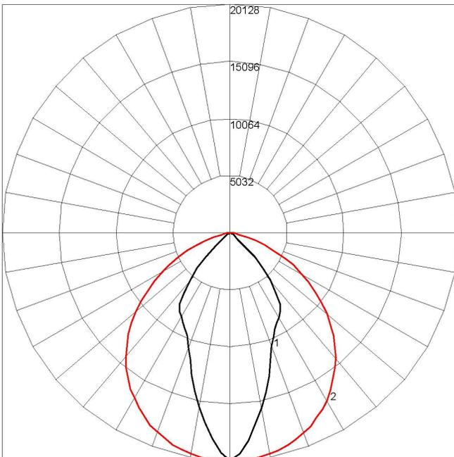
Maximum Candela = 20128.4 Located At Horizontal Angle = 85, Vertical Angle = 2.5
