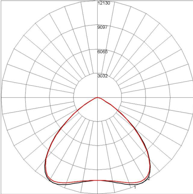
Maximum Candela = 12129.5 Located At Horizontal Angle = 0, Vertical Angle = 27.5
