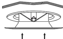
Gently push up the LED downlight until trim is flush with the ceiling. Ensure no wires are exposed. **Turn on power.**
