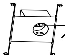
Screw adaptor into socket in recessed housing.
