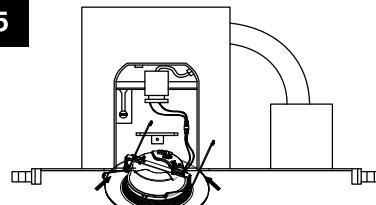
Gently squeeze together the torsion springs of the LED trim and insert into the recessed housing.
