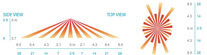
1. Sensors with Microphonics™ provides overlapping detection of human activity over the complete PIR coverage area. Advanced filtering is also utilized to prevent non-occupant noises from keeping the lights on.
