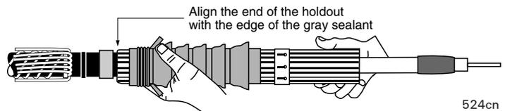
Slide the termination completely off the holdout using a twisting and pulling motion as shown.
