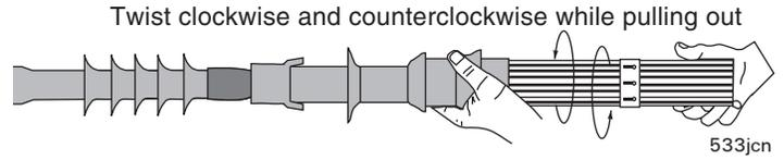
Using the pull tabs, pull the flip-back portion away from the main termination, at the same time working the first two fingers of each hand between the flip-back and main termination. Pull the stretched out flip-back over the sealant.
