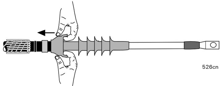
After installation, gently slide the termination so that the end aligns with the edge of the marker tape installed in step 5. Make sure the termination length is in accordance with the dimensions shown.
