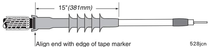
Having positioned the termination, now wrap one layer tape sealant over the end of the termination and 1/4" (6mm) onto the cable insulation as shown.
