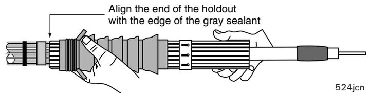
Slide the termination completely off the holdout using a twisting and pulling motion as shown.
