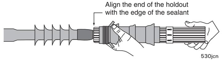
Slide the termination completely off the holdout using a twisting and pulling motion as shown.
