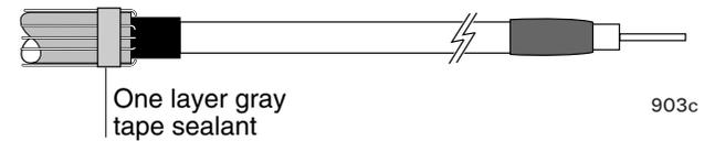
Wrap one layer of gray sealant over the wires and 1st layers of sealant.
