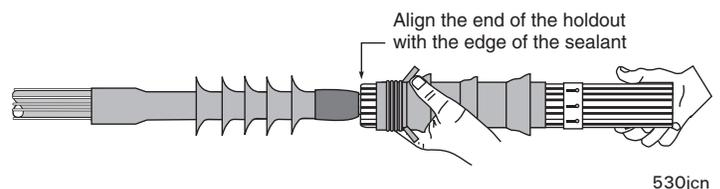
Slide the termination completely off the holdout using a twisting and pulling motion as shown.
