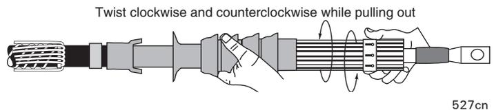
Using the pull tabs, pull the flip-back portion away from the main termination, at the same time working the first two fingers of each hand between the flip-back and main termination. Pull the stretched out flip-back over the cable jacket and sealant.
