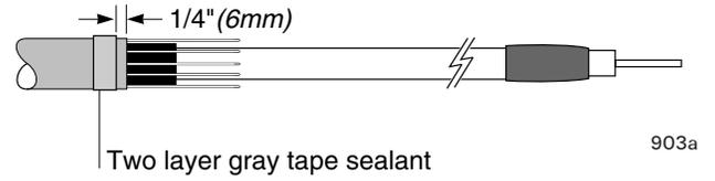
Without crossing, fold back neutral wires over the cable jacket cutback and press into the sealant.
