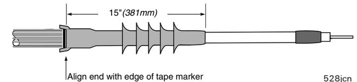
Having positioned the termination, now wrap one layer tape sealant over the end of the termination and 1/4" (6mm) onto the cable insulation as shown.
