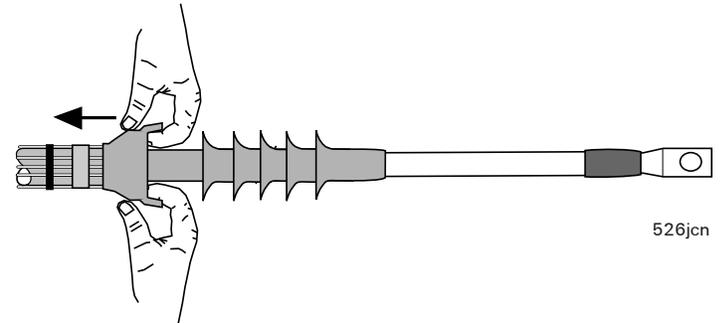
After installation, gently slide the termination so that the end aligns with the edge of the marker tape installed in step 5. Make sure the termination length is in accordance with the dimensions shown.
