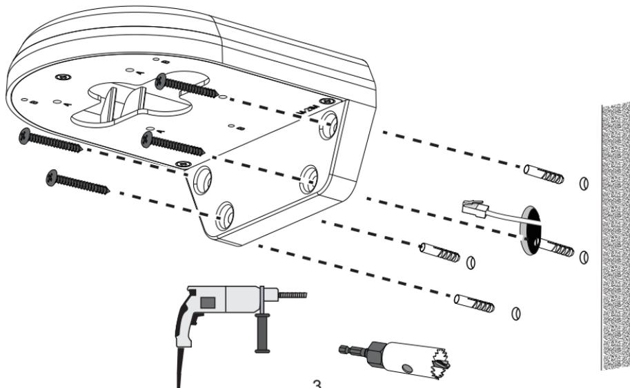
3. Route an Ethernet cable through the wall and the bracket. Install the waterproof components around the Ethernet cable.
