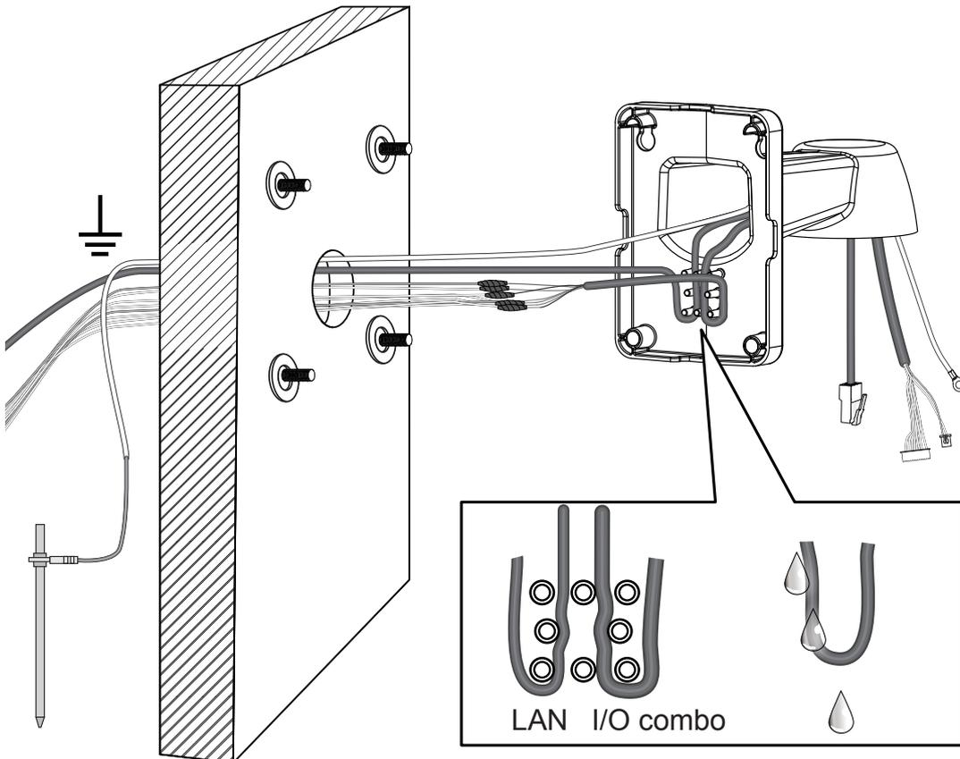
6. Secure the bracket to wall using a crescent wrench.
