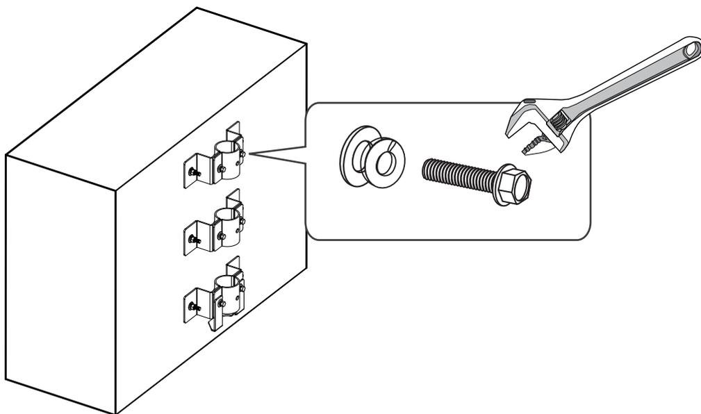
5. Install the AM-529 adapter to the parapet pipe.
