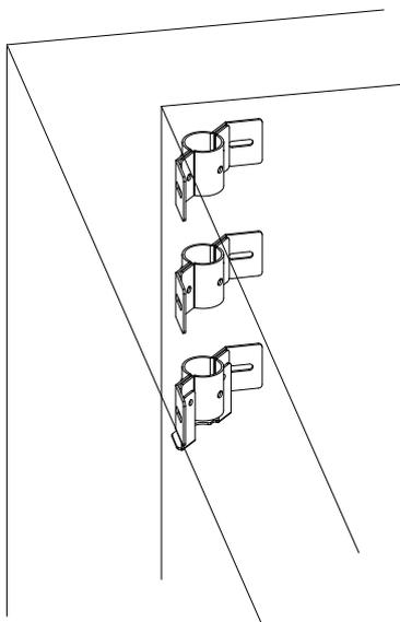
4. Use a crescent wrench to secure the outer brackets to the brackets on the wall using the M8x25 hex bolts and washers. Do not completely tighten the bolts yet! When the speed dome is installed to the mount pipe, it needs to be swiveled out to the desired position.
