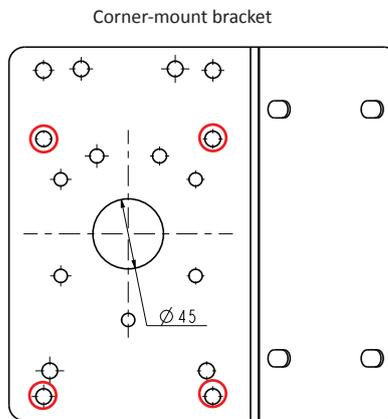
2. Align the top mounting plate with the center of the AM-21C bracket.
