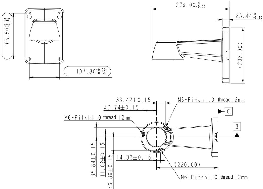
1. The mounting hole definition is illustrated below. The same mounting hole pattern apply to all pole-mount and corner-mount brackets.
