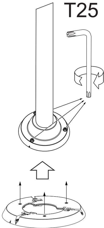
Note the front indicators indicate the default front side for the camera. Install the mounting plate with the orientation you prefer.
