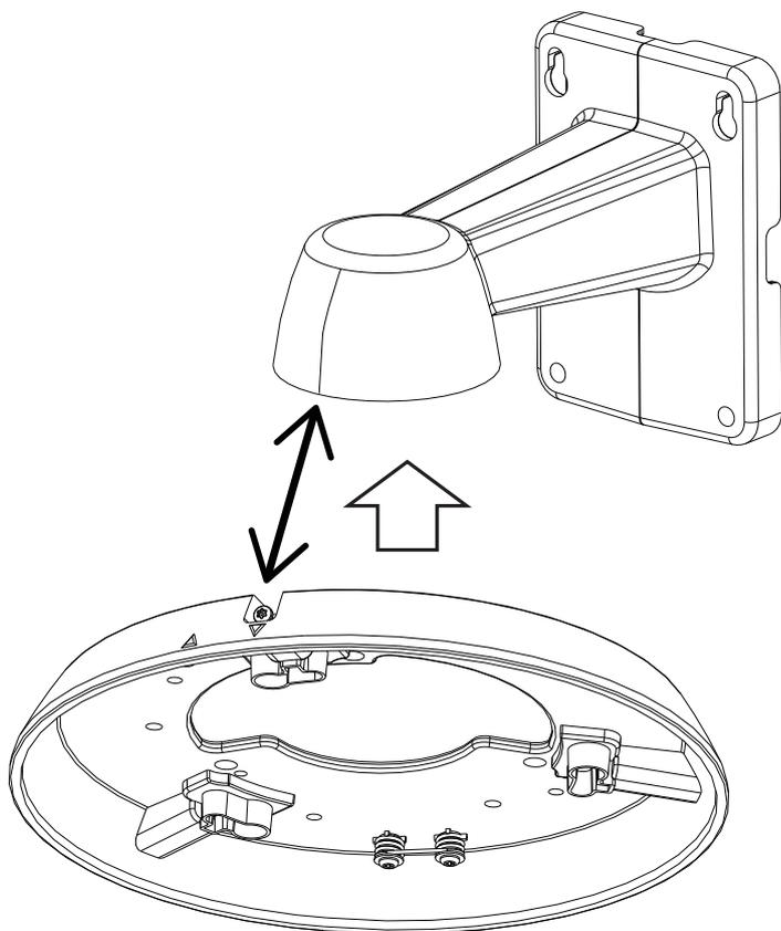
8. When aligned, secure the mounting plate to the AM-21C by driving 3 screws.
