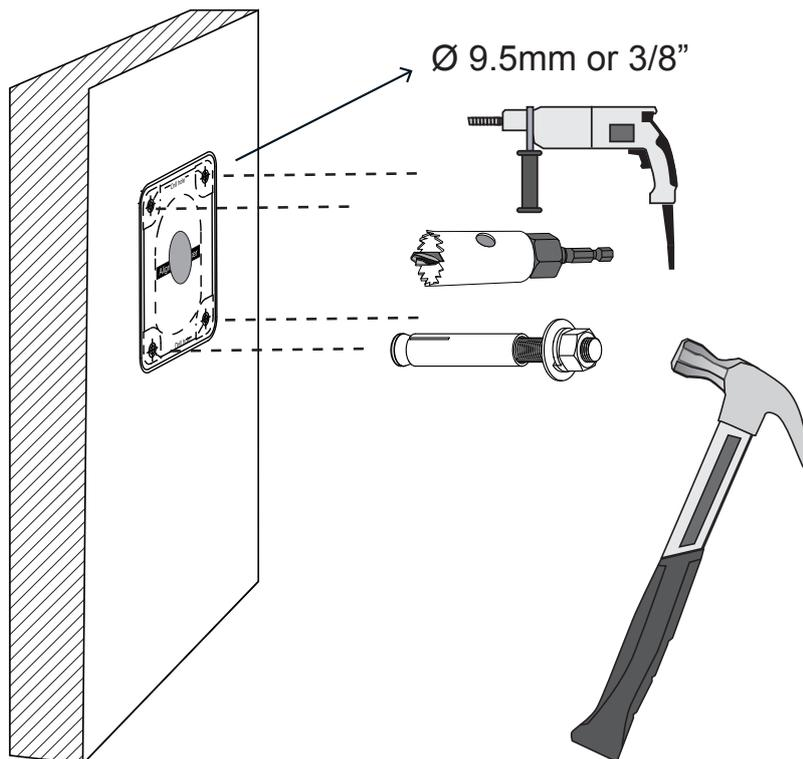
3. Remove the hex nuts, washers, and leave one washer on each of the threaded poles.
