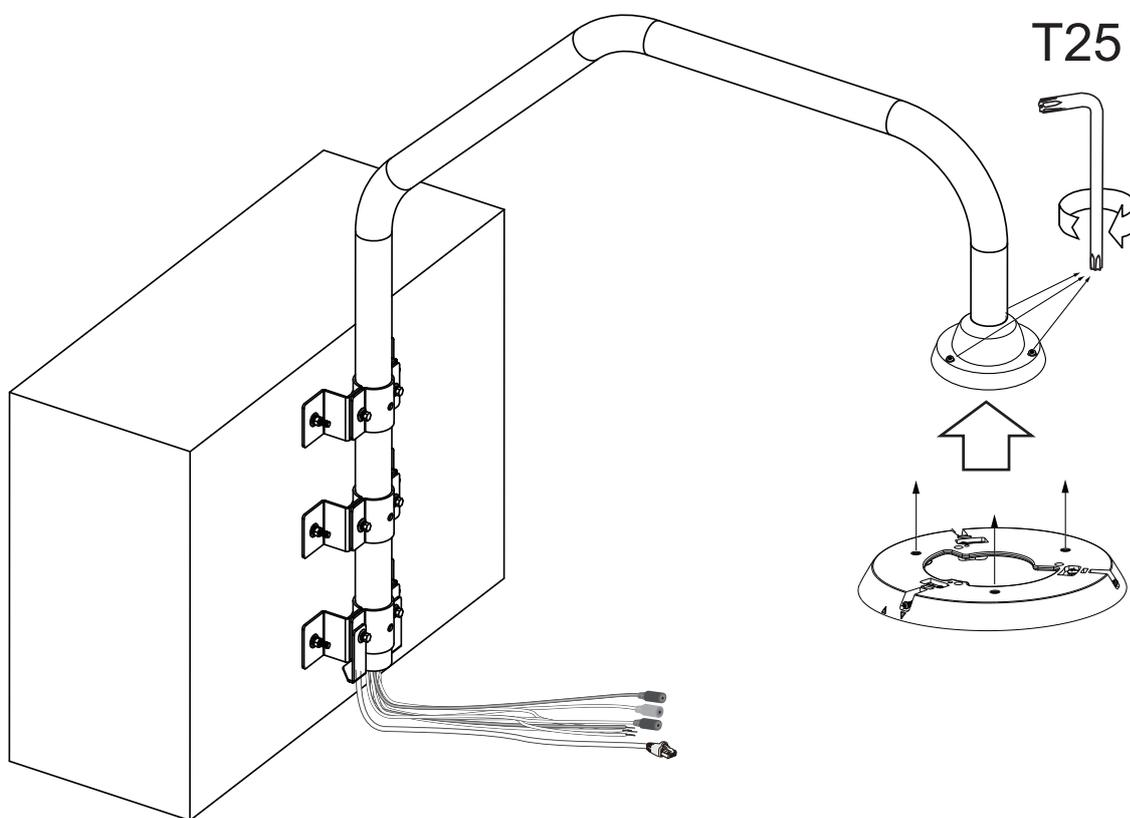
10. Swivel the pipe arm outwards to the opposite position. Use the M8 x70 bolts to secure the pipe arm to the brackets. You also need to tighten the M8 x25 bolts between the inner and outer brackets.
