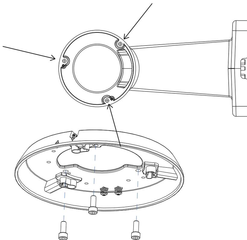
7. Install the camera to the AM-21C and the junction box. Refer to the camera's documentation for the rest of the installation details.
