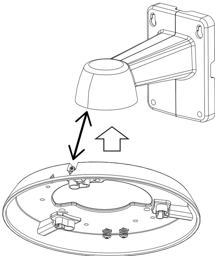
3. When aligned, secure the mounting plate to the AM-21C by driving 3 screws.
