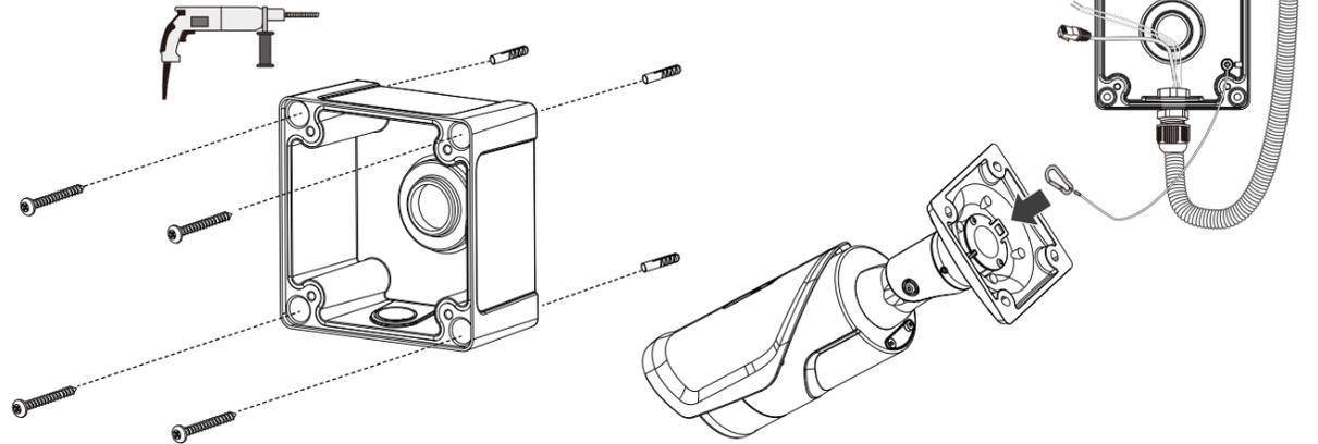
The drawing takes IB9365 as an example. The combo cables are not shown here for the simplicity reason.
