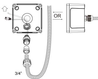
Attach the included alignment sticker to a preferred position. Drill holes on the wall and install the junction box. If space behind the wall allows, you may also pass cables through the
