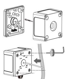
Install the camera using the corresponding mounting holes with the included hex socket screws.
