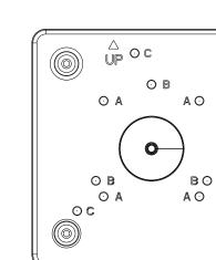
Pass the camera's Ethernet cable through the center hole of the box and the rubber seal.
