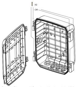
Pass the Ethernet and I/O combo cables through the M20 cable glands, and into the cabinet. You may need to open the cabinet. Secure the camera mount bracket (here a speed dome bracket is shown) to the cabinet. You can then install the camera. Refer the camera's documentation for information.
