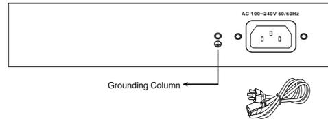
The switch already comes with lightning protection mechanism. You can also ground the switch through the PE (Protecting Earth) cable of AC cord or with Ground Cable.
