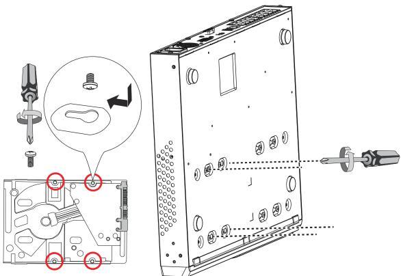
6. Secure the hard disks to the mounting positions in the chassis with its label side facing up, and the connectors facing the inside of the chassis. The sample drawing below shows the
