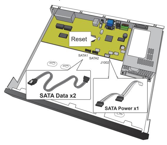
4. Connect the SATA power and SATA data cables to the hard disk drives.
