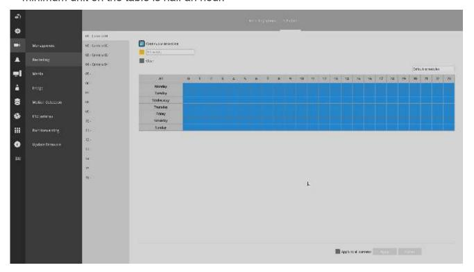
3. You may also use the scheduler tool on the right to facilitate the process. You can select a condition checkbox, and then select the All day, Work hour, Off duty, Working day, Weekend options to apply a time selection.
