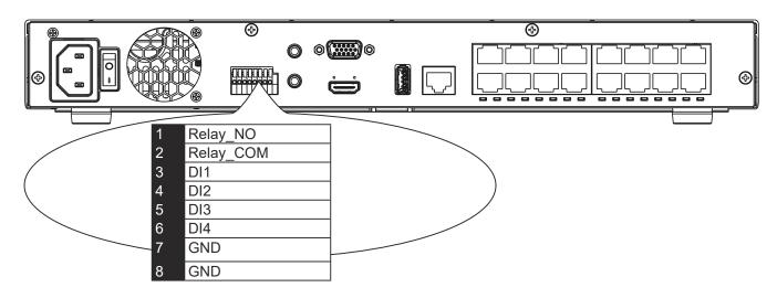
The GND are common ground for the DIs.
