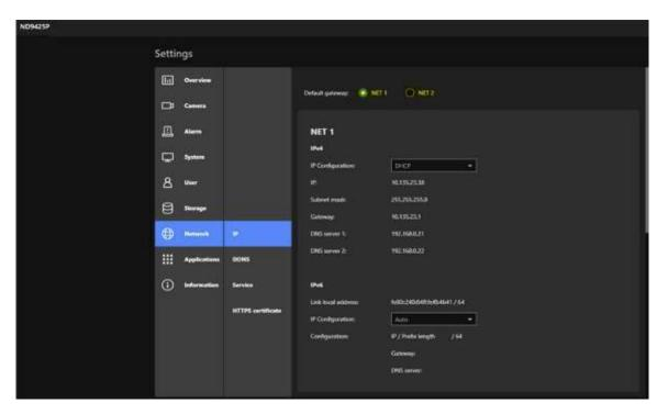
You can select DHCP as the method for cameras to acquire IP addresses, or you can manually configure static IPs for a single or all cameras. Although the NVR can remember the MAC addresses of cameras, if IPs are changed under the DHCP configuration, your NVR may still fail to connect the cameras. Please consult your network administrator for details about network settings.
