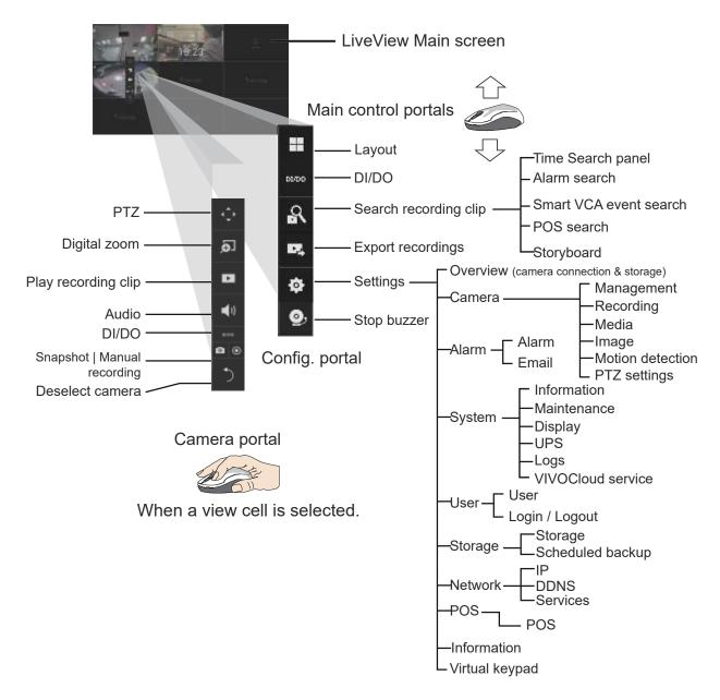
After you finish configuring using a Camera portal, click again on the camera view cell to reveal the main control portals.
