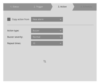
If events of different importance are issued at the same time, e.g., one major and one minor event, system will ignore the minor event and sound the buzzer tone for the major event only. The buzzer can be sounded either by the Alarm actions or the system events. If Alarm actions and system service events occur at the time, Alarm actions have the higher priority.
