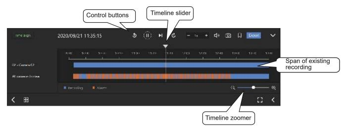
The time slide bar enables quick skimming through the recording. Its functional buttons are described as follows:
