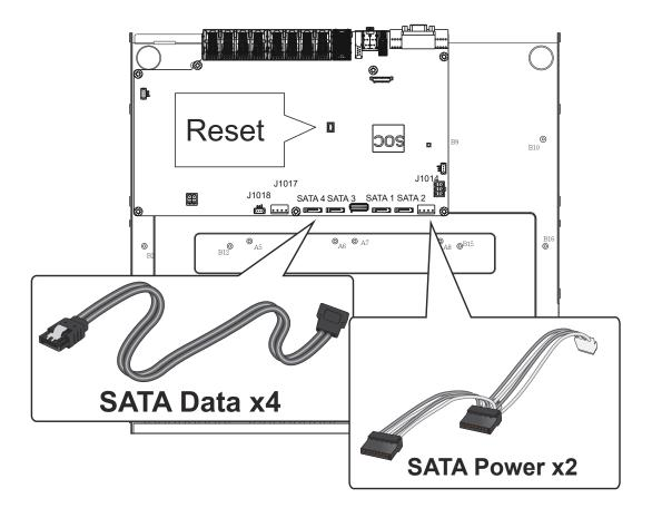
5. Connect the SATA power and SATA data cables to the hard disk drive.
