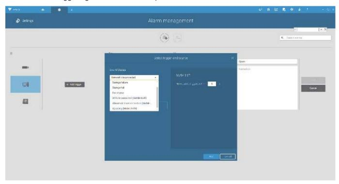
Configure the corresponding action, and proceed with the rest of the configuration. When an event is triggered, such as GPS signal loss, or exceptional G-force is detected, an event message will prompt on screen. You can also search the past alarms to find an event.
