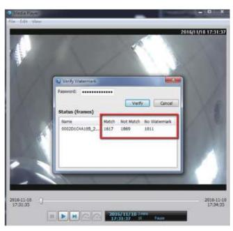
Enter the password to verify. If the Not match value is 0, the video is the original and has not been tampered with.
