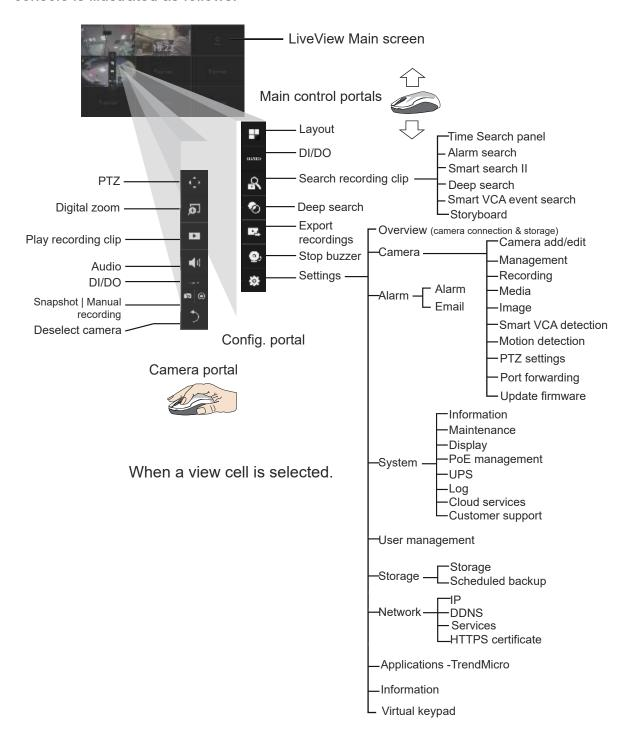
After you finish configuring using a Camera portal, click again on the camera view cell to reveal the main control portals.
