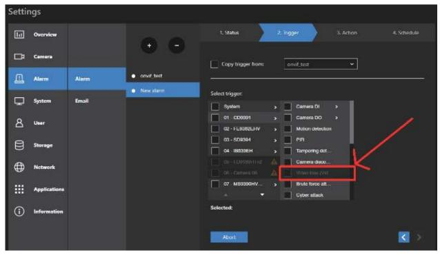
You can also find the "RAID degraded" option, which can be triggered when RAID is corrupted or undetected. In addition, the "Video loss (for video server only)" option (see the above red box) will be available if connecting to a video server.
