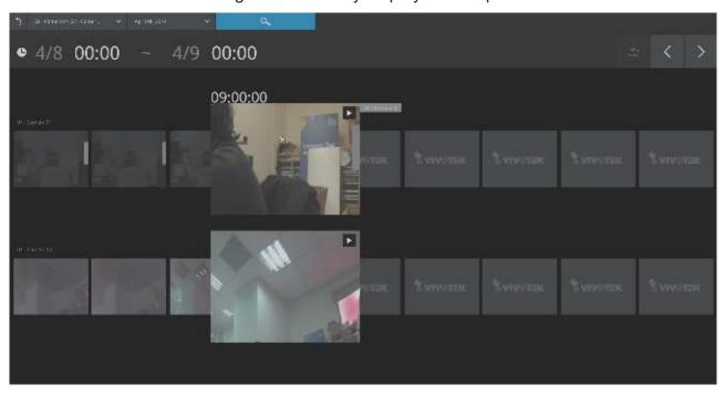
The detailed search is based on a narrow-down criteria. The search begins from a 24-hour time span, and then moving in to a 4-hour, 1-hour, 10-minutes, and 2-minutes span. When the screen displays a 24-hour span, each snapshot represents a 3-hour time span.
