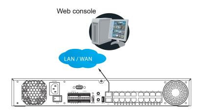
Note that when accessed over the network, the total streaming throughput is 24Mbps.
