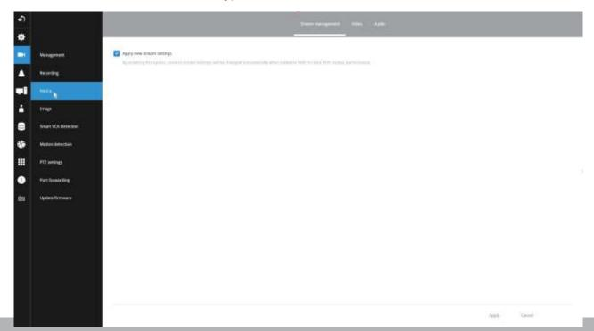
The NVR adaptively selects to display a video stream of a different resolution when it is displaying on a smaller view cell or a full screen.
