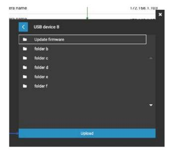
The Batch upload function allows you to update the firmware of multiple cameras. The firmware update can take place on up to 8 cameras at a time. The Waiting... message will display for cameras that are waiting for the update to take place.
