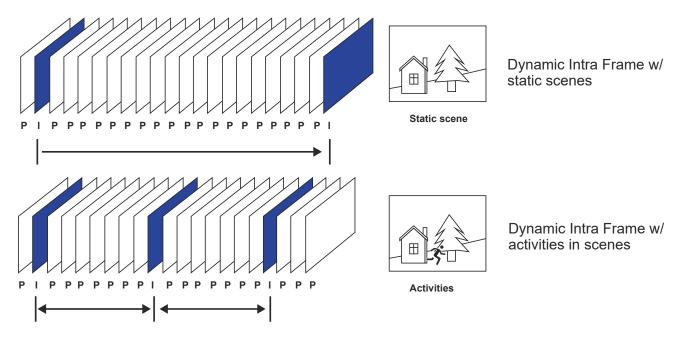
■ Smart codec effectively reduces the quality of the whole or the non-interested areas on a screen and therefore reduces the bandwidth consumed.
