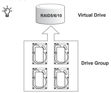
Our default recommendation is to combine 4 hard drives into 1 drive group. The capacities of these drives will be utilized to form 1 Virtual Drive. If all 8 drive bays are populated, you can create 2 Virtual Drives. A 4-member Virtual Drive can receive the video feeds from 32 to 128 cameras. You can also create one 8-member Virtual Drive to receive the video feeds from 32 to 128 cameras (CH, or channels.)
