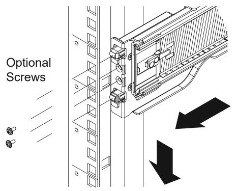
5. Extend the rails as necessary, and repeat the previous step to hang the slide rails to four rack posts.
