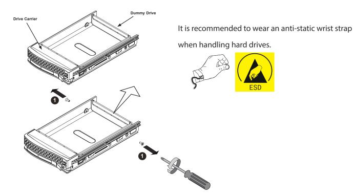
3. Install hard drives by driving screws from the sides. When done, gently install the drive trays into the chassis.
