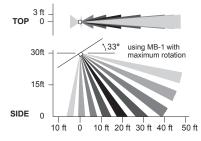
Coverages shown are maximum and represent half-step walking motion. Under ideal conditions with no barriers or obstacles, coverage for half-step walking motion with the standard lens can reach up to 2000 ft2, while coverage for typical desktop activity can reach up to 1000 ft2. When using the CX-100/105-1 or -3 lens, motion moving toward sensors will begin to be detected at 55 to 60 feet.
