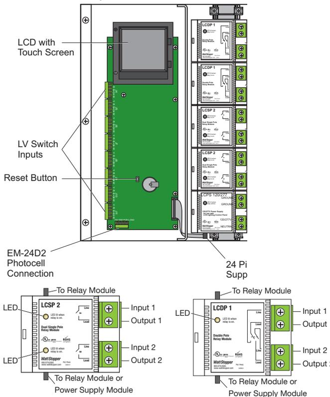
Relay modules can be mixed and matched to configure the LC8 for a variety of single-pole and double-pole lighting control applications.
