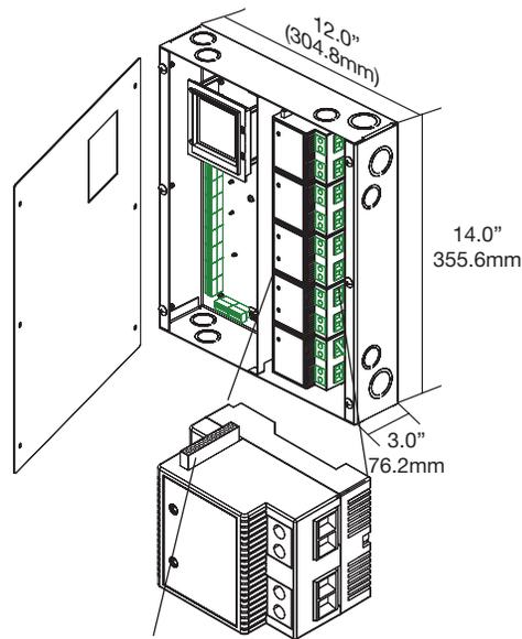
Modules clip onto DIN rail, and plug to panel power supply and each other via integral connectors.
