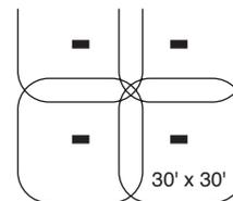
Typical layout for open office space would be to place UT-355-3 sensors so they control zones that overlap. For partitioned spaces, a typical zone is about 25' x 25' with an overlap on the coverage up to 30' x 30'.
