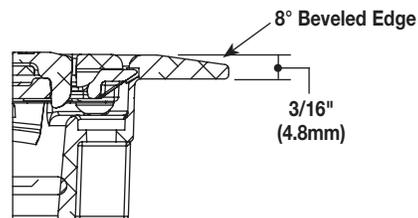
NOTE: All surface style poke-thru devices come with a transition angle to aid in the change in floor elevation.
