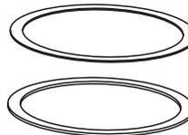
**Tile Shim –** Used for floor coverings greater than 3/16" (4.8mm). The 8TS will allow the top surface of the cover to be flush with the finished floor. Includes: six (6) 1/16" (1.6mm) thick shims. Up to a total of 3/8" (9.5mm) of adjustment.
