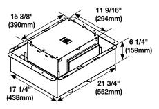
**8-Gang Fire Classified Floor Box** – Pre-assembled installation ready floor box has been designed to be installed in above grade concrete floors while maintaining the fire classification of the floor. This box is classified to be used in 1-, 1 1/2-, 2-, or 3-hour fire rated floors. Designed to accept standard size wall plates. **Box comes complete with all components needed for initial installation.**
