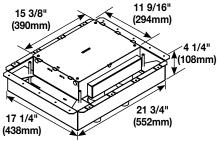
**6-Gang Fire Classified Floor Box** – Pre-assembled installation ready floor box has been designed to be installed in above grade concrete floors while maintaining the fire classification of the floor. This box is classified to be used in 1-, 1 1/2-, 2-, or 3-hour fire rated floors. Designed to accept standard size wall plates. **Box comes complete with all components needed for initial installation.**
