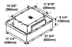
**8-Gang Fire Classified Floor Box** – Pre-assembled installation ready floor box has been designed to be installed in above grade concrete floors while maintaining the fire classification of the floor. This box is classified to be used in 2-hour fire rated floors. Designed to accept standard size wall plates. **Box comes complete with all components needed for initial installation.**
