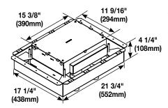
**6-Gang Fire Classified Floor Box** – Pre-assembled installation ready floor box has been designed to be installed in above grade concrete floors while maintaining the fire classification of the floor. This box is classified to be used in the 2-hour fire rated floors. Designed to accept standard size wall plates. **Box comes complete with all components needed for initial installation.**
