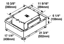
**10-Gang Fire Classified Floor Box** – Pre-assembled installation ready floor box has been designed to be installed in above grade concrete floors while maintaining the fire classification of the floor. This box is classified to be used in 2-hour fire rated floors. Designed to accept standard size wall plates. **Box comes complete with all components needed for initial installation.**
