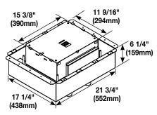
**8-Gang Fire Classified Floor Box** – Pre-assembled installation ready floor box has been designed to be installed in above grade concrete floors while maintaining the fire classification of the floor. This box is classified to be used in 1-, 1 1/2-, 2-, or 3-hour fire rated floors. Designed to accept standard size wall plates. **Box comes complete with all components needed for initial installation.**
