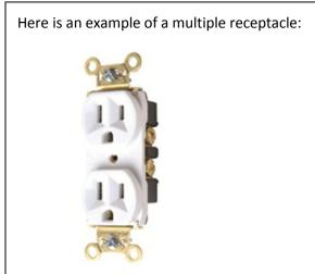
In accordance with Section 18-27-210.21(b)(1), If a single receptacle is installed on a branch circuit, it shall have an ampere rating of not less than that of the branch circuit. Also, Section 18-27-210.21(b)(3) states that a branch circuit supplying two or more receptacles or outlets shall use receptacles that are rated in accordance with Table 18-27-210.21(b)(3), shown below. For a 20-ampere circuit, this table allows either a 15-ampere or a 20-ampere receptacle to be used.
